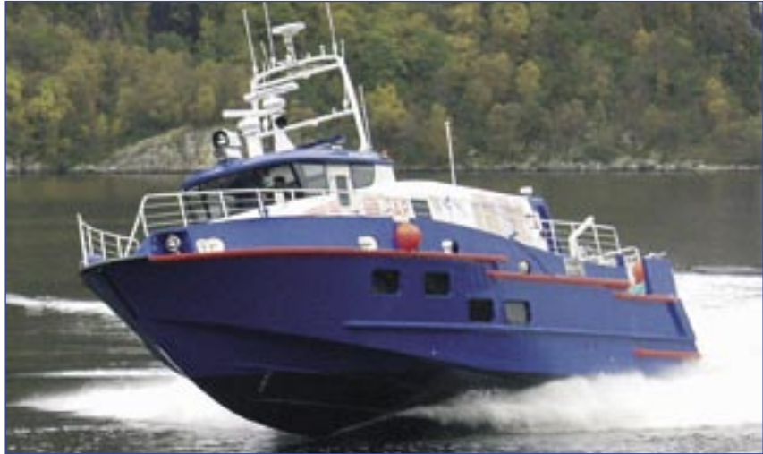
The core infused ambulance boat that has just been 'launched' by Brødrene.
