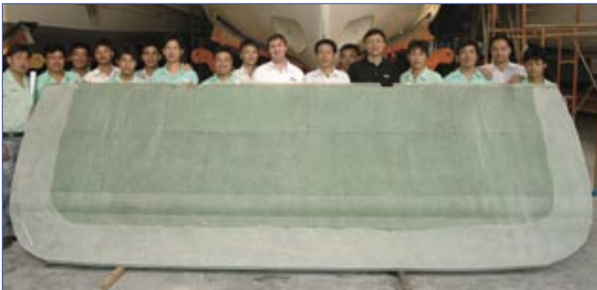
The Jet-Tern 'infusion team' plus Todd Henry and Forest Song from DIAB with the infused bulkhead.
