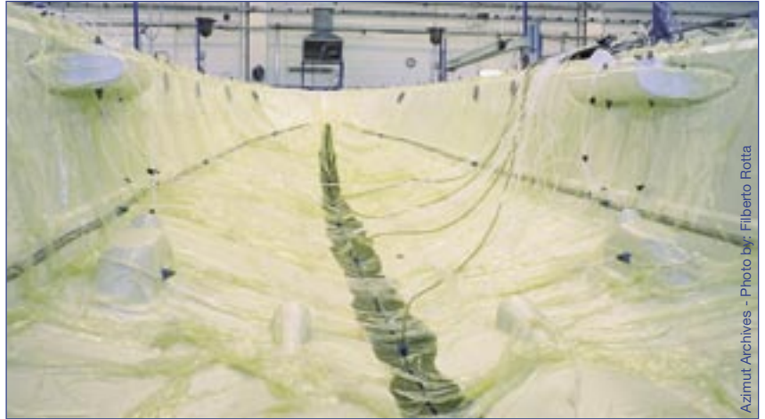
The production of an Azimut hull using DIAB Core Infusion Technology™.
