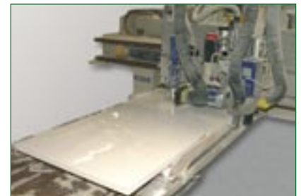
A Fib-R-Dor under construction.
