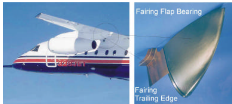
Fig. 4: CFRP Panelling elements on the engine pylon of the Do 328 Jet
